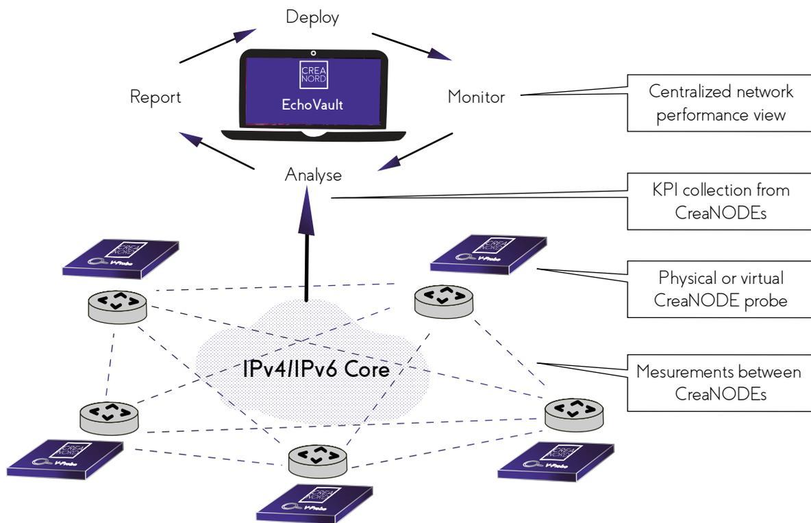
Figure 1 Creanord solution for IP Core monitoring
